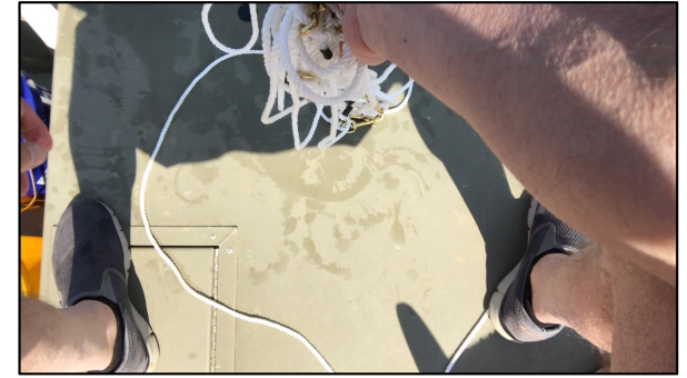
Method 1: let the anchor line gather where, then toss the gathered anchor line overboard to sort itself out
