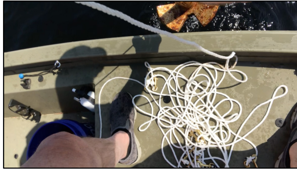
Haul the anchor up ... careful not to drag the anchor fastener across the gunnel (it can catch and drop the anchor)
