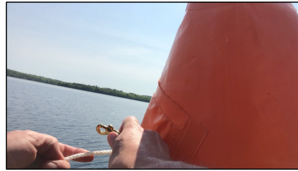
Disconnect anchor line from the mark (the other end is still attached to the anchor)
