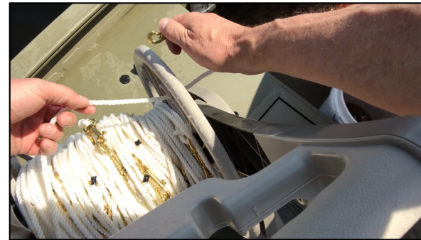
When done with the anchor line, loop it through one of the ends of the spool and clasp the line upon itself
