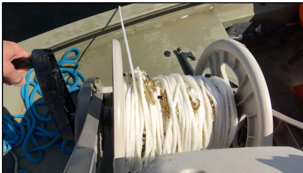
Disconnect the anchor line from the anchor and throw the loose end of the anchor line overboard and the reel in the anchor line
